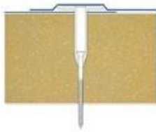
Incorrect installation Too loose pressure plate tube
